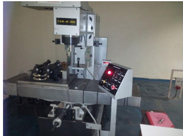
Fig: 2. Friction stir welding / processing machine (Central workshop, Delhi Technological University)
